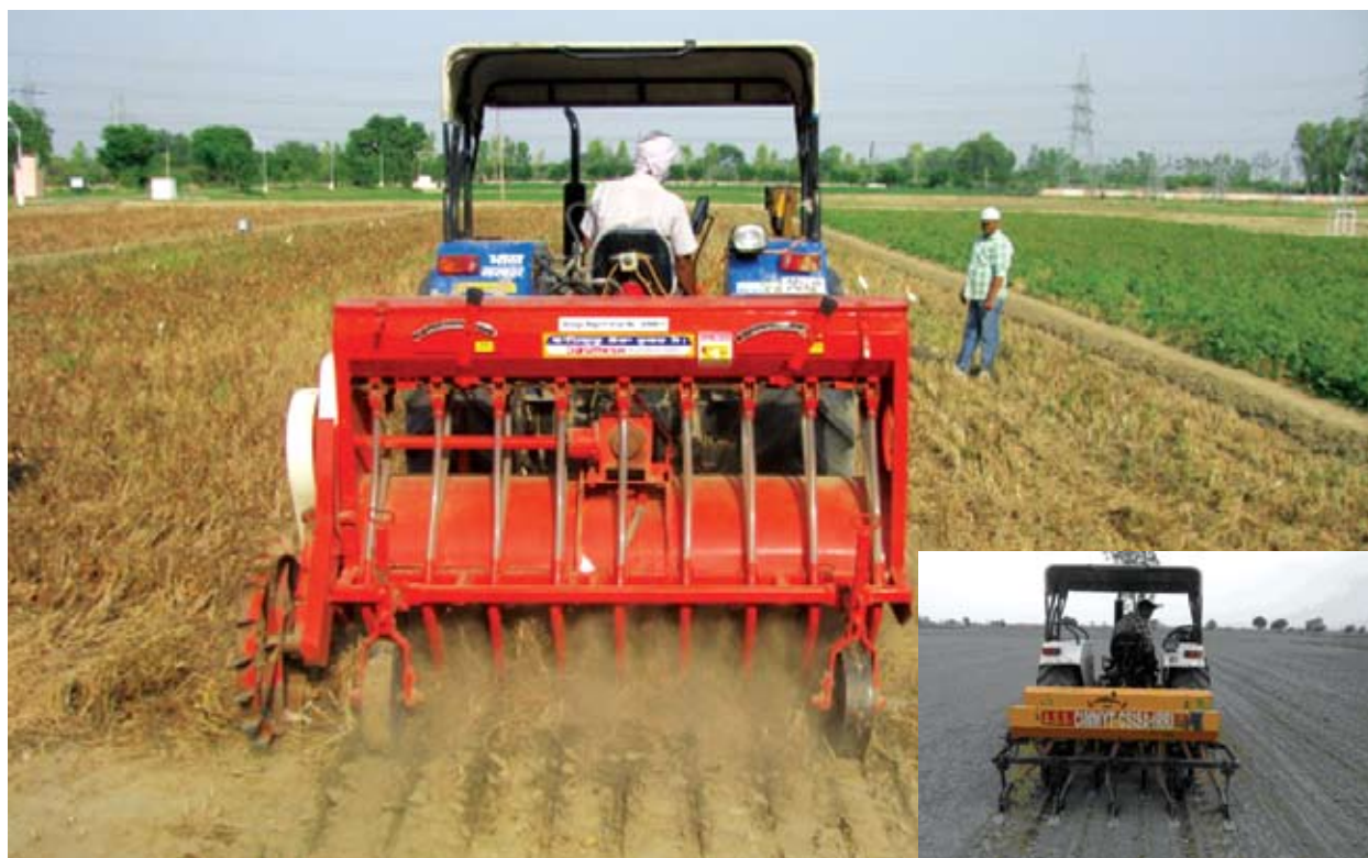
Figure 5. Different machines which can be used for seeding rice: a) Multi-crop planter with inclined plate seed metering system, b) turbo happy seeder
