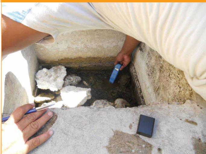
Ground water well where salinity is being measured.
